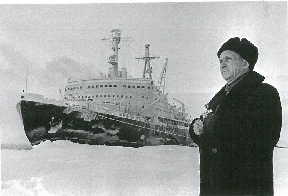
*The early ice-breakers that were unable to help the Chelyuskin in the early 1930's have long been superseded by modern ships that can break through every ice barricade that the Arctic Ocean can devise. This powerful nuclear-powered ice-breaker, Lenin, went into Arctic service in 1959. Today, even larger vessels of similar size and greater power such as the Yamal, can even take international tour groups to the North Pole.*
